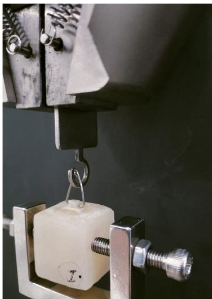
Figure 5: Sample placed in universal testing machine
