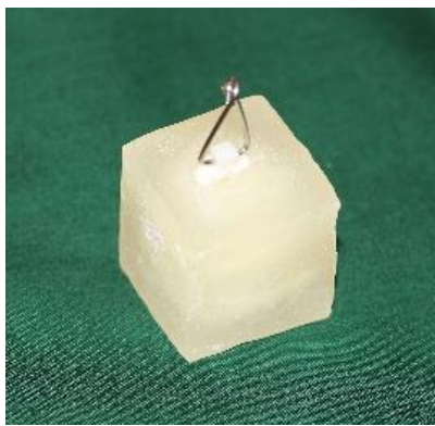
Figure 4: composite rod with incorporated triangular shaped wire on prepared tooth surface
